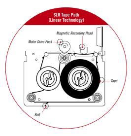
Linear recording technology represents a more efficient cartridge and drive design that reduces tape stress, ensures data integrity and increases drive and cartridge reliability.
